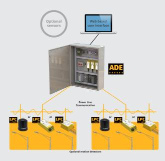
In a TLACS lighting control solution, the LPC Twist communicates two-way over powerline, using the electrical system that supplies the luminaires with electricity. This means that you don't have to dig to add wires for the control and monitoring of the luminaires.
